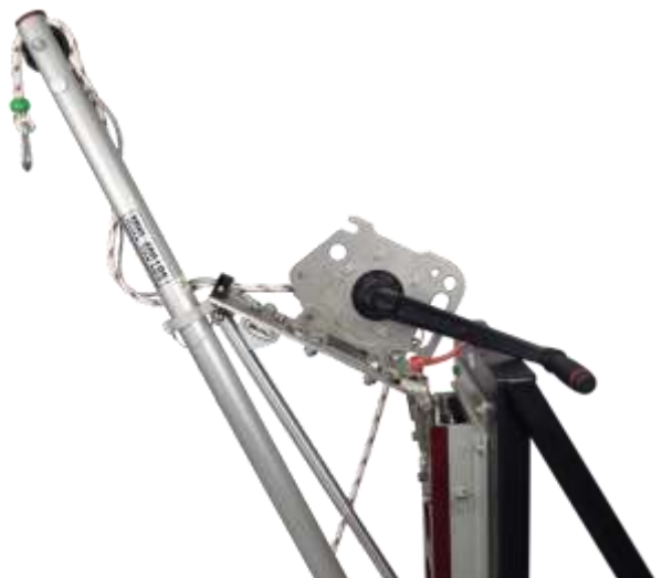
Image L13 – Boom folded up and mounted
