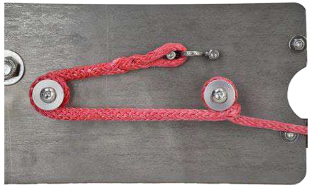
Image F15 Tension line wrapping finished
