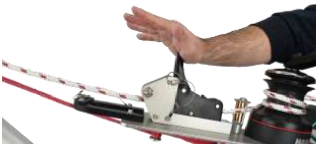
Image F8 Line released with hand on brake
