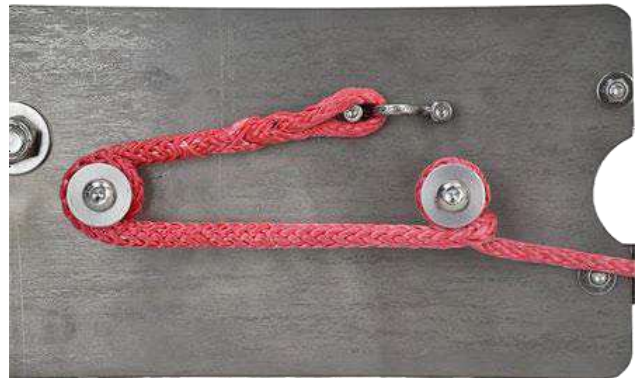
Image H15 Tension line wrapping finished
