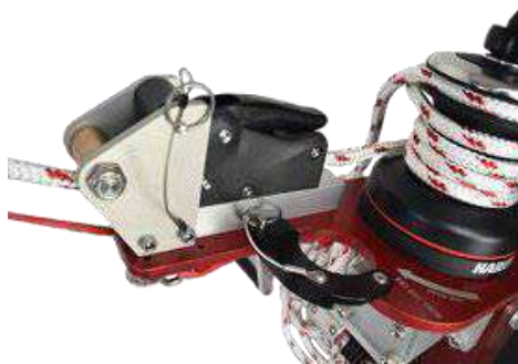
Image J31 Line brake closed; line wrapped in winch jaws & ready to lift
