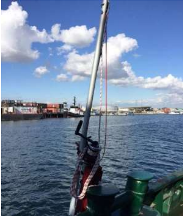
Image J29 Rescue davit attached & ready to deploy
