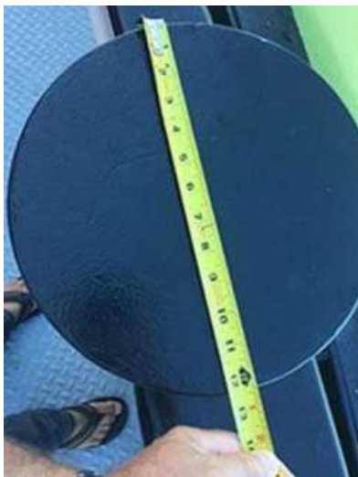
Image G5 Measure bitt diameter
