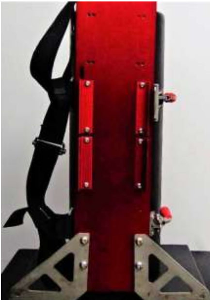
Image E7 Quad foot version shown. For shorter bits, the top red feet and band attachments have been moved down to the lower sets of holes. All 4 feet would also be moved closer for a bit diameter less than 8 1/2"
