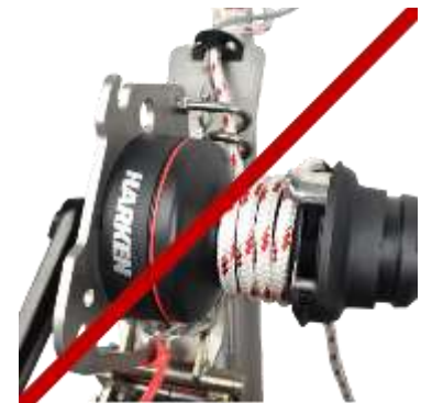
Image L16 – WRONG: Lift line is not over the tailing arm, compare to L14
