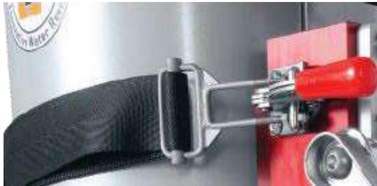
Image J22 Top strap with clamp ready to be closed
