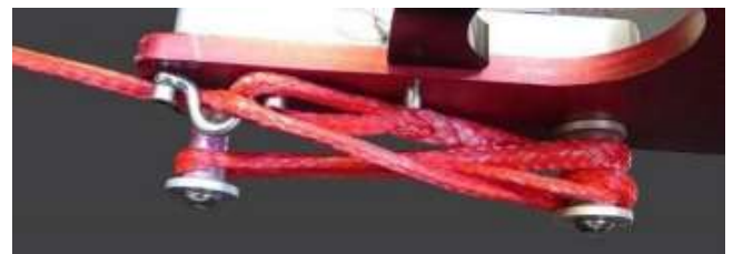
Image K15 Eye strap refastened with the tension line running through it
