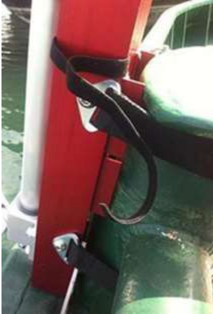
Image J3 Depicts how the Rescue Davit should fit, not bottoming out and touching the bitt between the rear angle feet
