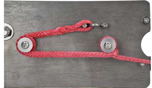
Image G31 Tension line wrapping finished
