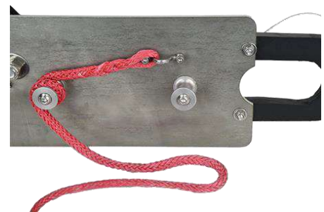
Image G29 Tension line start rear button only
