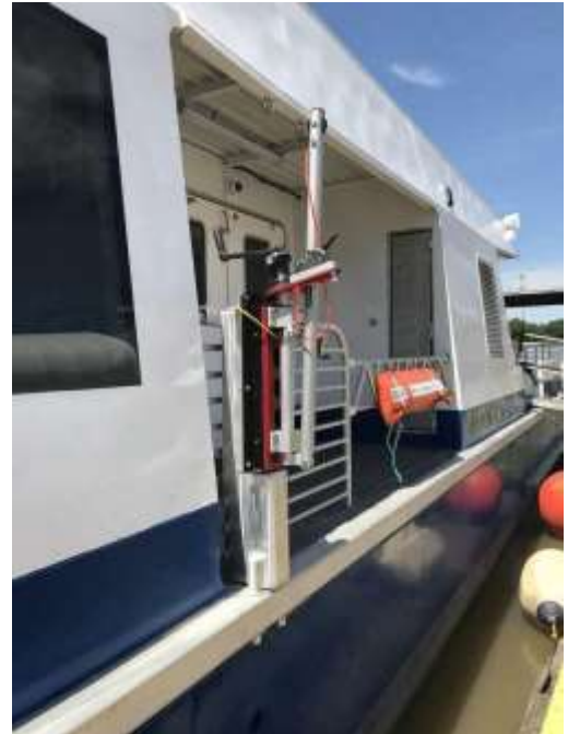
Image K18 Flat Mount rescue davit on a passenger ferry boat
