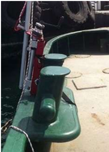
Image G9 Depicts a big top flange & how it was cut off to make the Rescue Davit work *7 Series shown – 5 Series mounting is identical*
