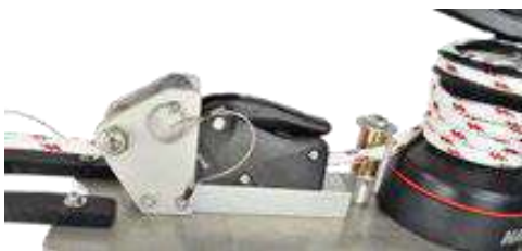
Image G34 Line brake closed, line wrapped in winch jaws and ready to lift
