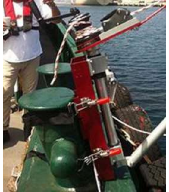
Image J4 A properly installed Bitt Mount Rescue Davit
