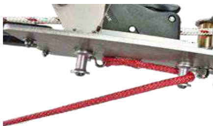
Image G28 Beginning wrap to adjust boom height angle
