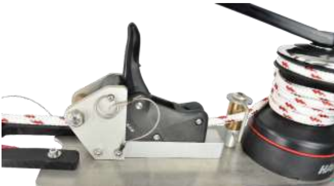
Image H6 Line brake open
