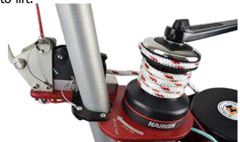
Image J21 Davit boom stowed and pinned
