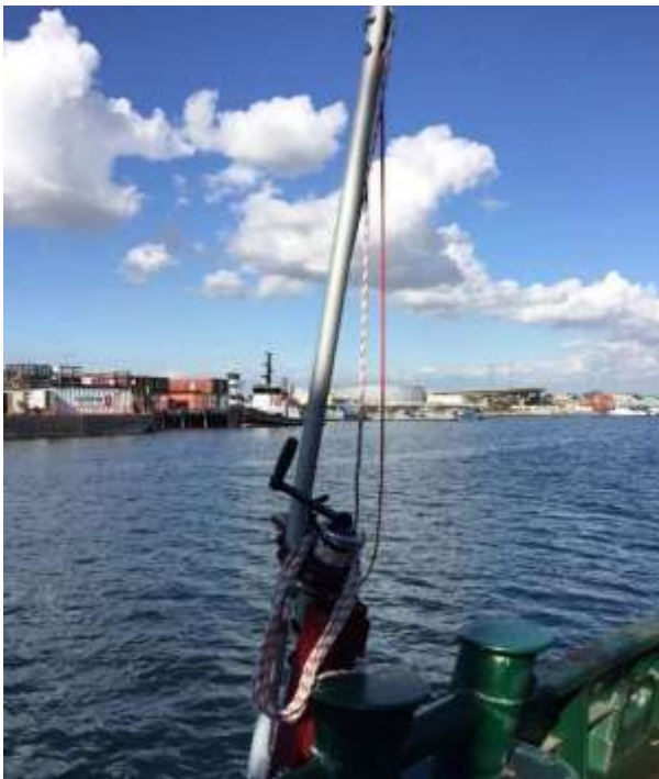
Image G32 Rescue davit attached & ready to deploy *7 Series shown – 5 Series bit attachment is the same
