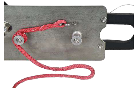
Image E25 Tension line start rear button only
