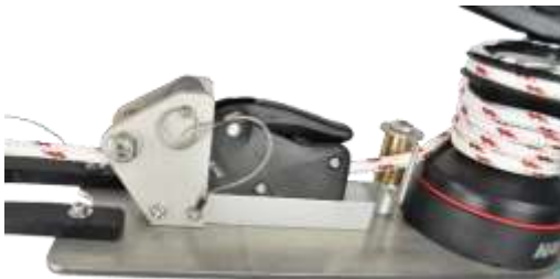
Image F19 Line brake closed; line wrapped in winch jaws & ready to lift
