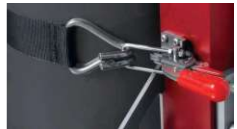
Image E13 Bottom hook in place
