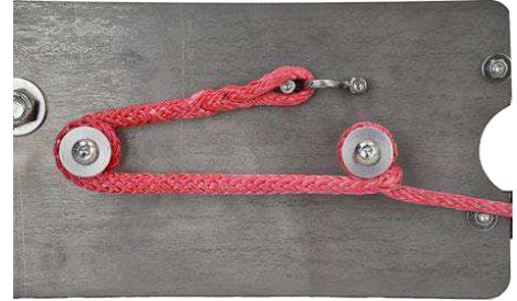
Image E27 Tension line wrapping finished
