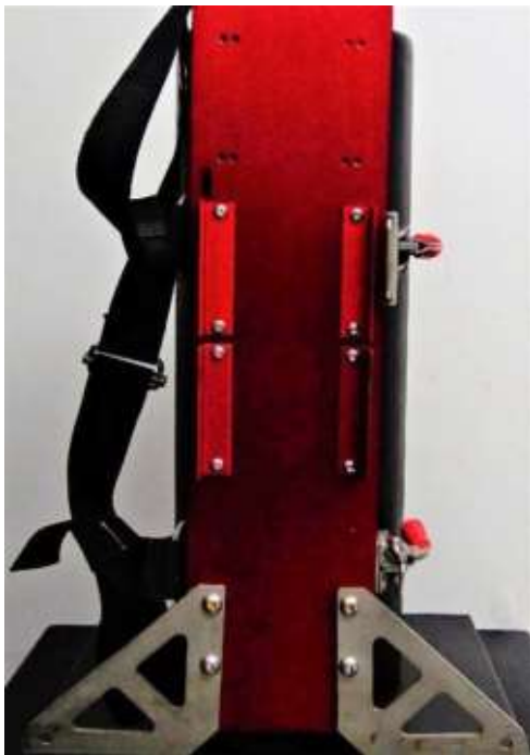
Image J7 Back feet, 4 feet version. For shorter bitts, the top red feet and band attachments have been moved down to the lower sets of holes. All 4 feet would also be moved down for a bit diameter less than 8 1/2"
