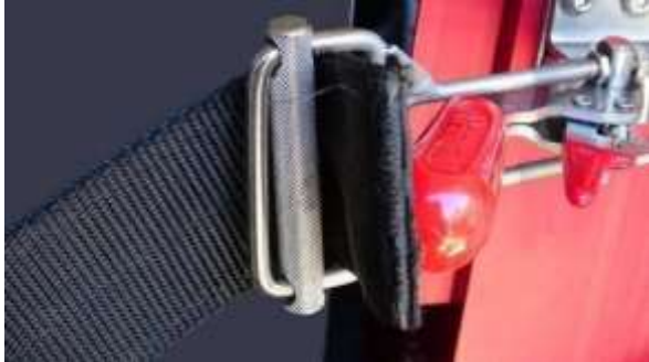
Image E9 Top buckle thread
