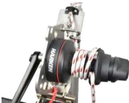
Image L14 - Correct way to load the winch, and ready
