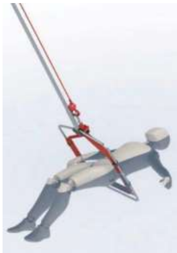
Image B10 Move pole down and hoop down to get under the other arm
