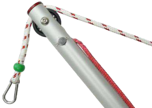
Image K5 Tension line around the pin inside of the boom. Cotter pin has been inserted and bent to secure in place.
