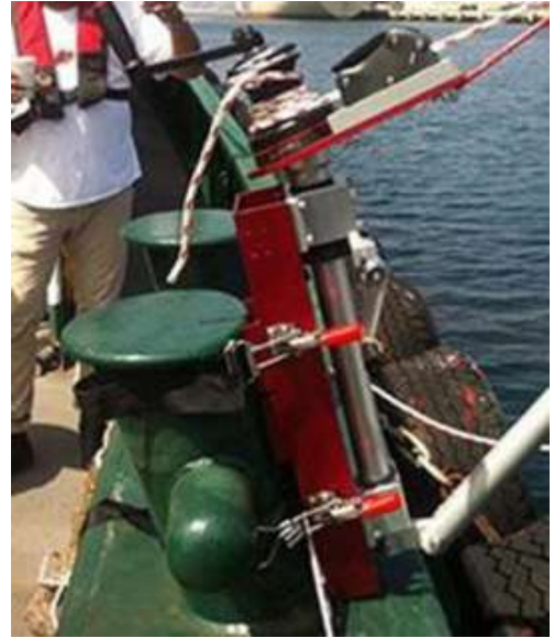
Image G8 A properly installed Bitt Mount Rescue Davit - *7 Series shown – 5 Series mounting is identical*
