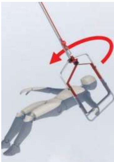
Image D10 Start under one arm, up to the arm pit and rotate hoop over the head
