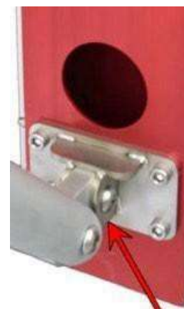
Image G20 Boom connected to davit base
