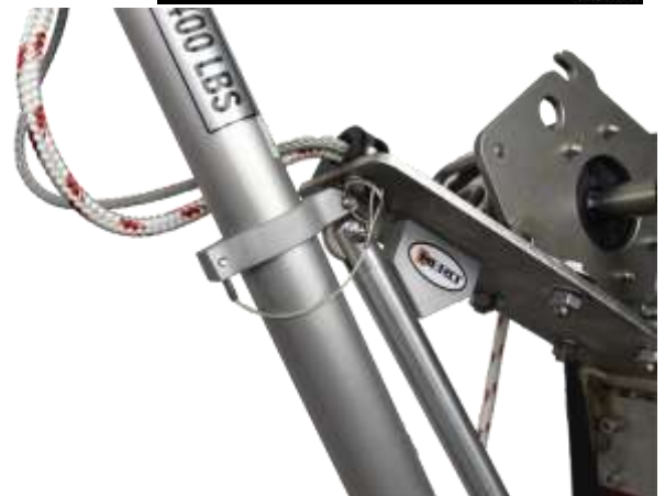
Image L10 – Close-up of davit folded up & pinned
