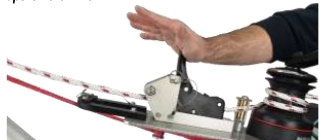
Image E31 Line brake open
