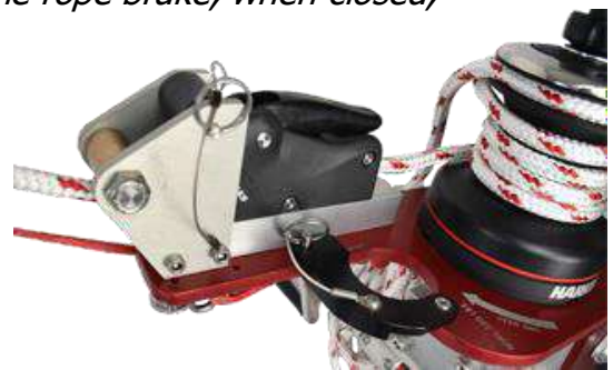
Image J19 Line brake closed, line wrapped, in the winch jaws. Tailed off the chrome tailing arm and ready to lift.
