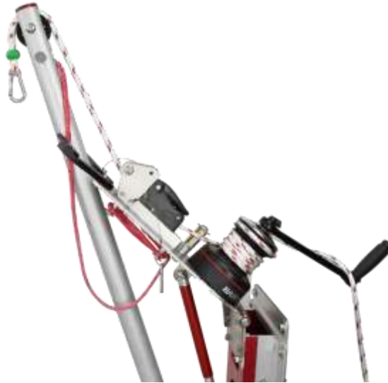
Image H21 Boom topped off to the end of the winch plate. Bring PIW back aboard
