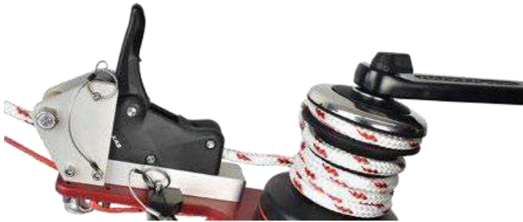
Image K6 Line brake open
