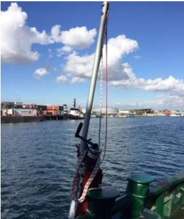
Image E28 Rescue davit attached & ready to deploy *7 Series shown – 3 Series bit attachment is the same
