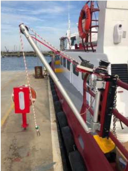
Image K17 Flat Mount rescue davit, on a crew boat, secured with stainless steel U bolts on a sturdy railing
