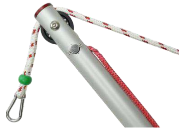
Image J17 Tension line around the pin inside of the boom. Cotter pin has been inserted and bent to secure in place.
