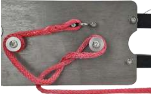
Image E26 Tension line putting two twists counterclockwise
