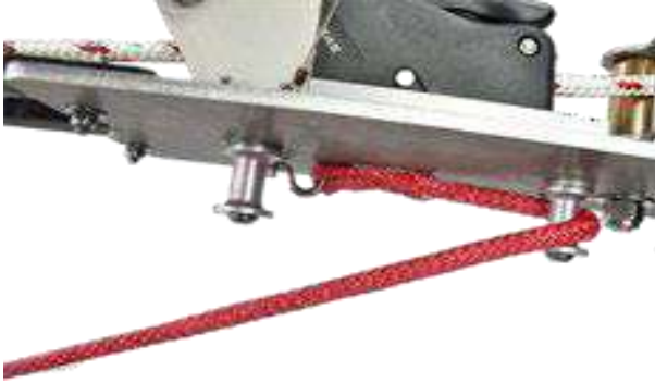
Image H12 Beginning wrap to adjust boom height angle
