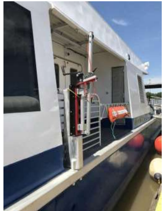
Image H18 Flat Mount rescue davit on a passenger ferry boat
