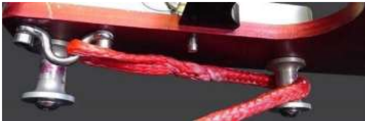
Image K12 Beginning wrap to adjust boom height angle
