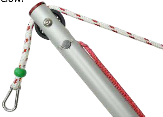
Image E17 Tension line around the pin inside of the boom. Cotter pin has been inserted and bent to secure in place.
