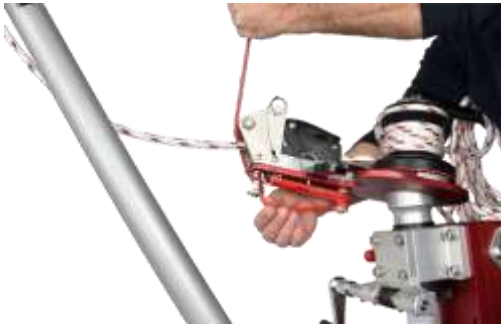
Image J24 Boom height adjustment, with davit securely attached to the bitt. Holding the red tension line, lift the boom to approximately to a 45-degree angle and wrap the red tension line around the tension line adjusting buttons found underneath the winch plate.
