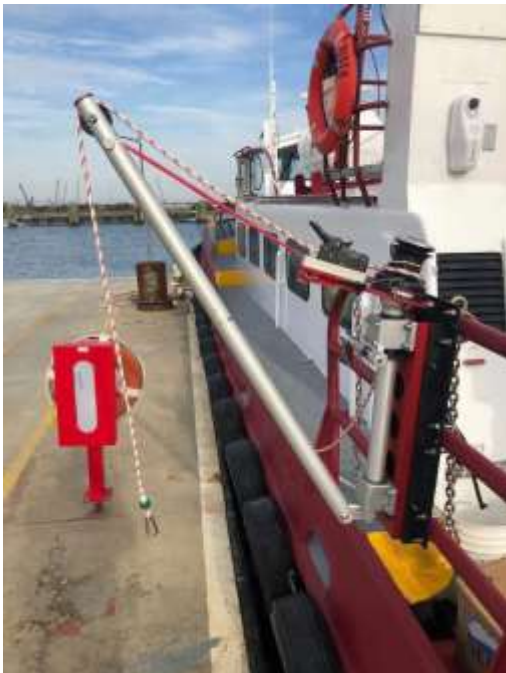
Image H17 Flat Mount rescue davit, on a crew boat, secured with stainless steel U bolts on a sturdy railing
