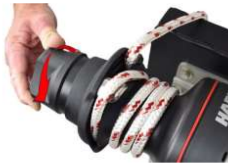
Image L15 - Twist the brake knob clockwise to ease line out slowly
