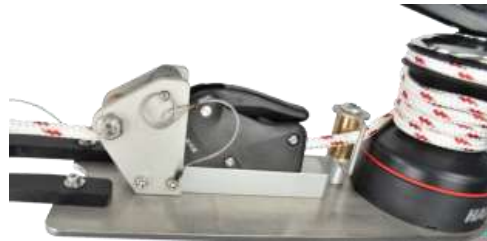
Image E19 Line brake closed, line wrapped, in the winch jaws. Tailed off the chrome tailing arm and ready to lift.
