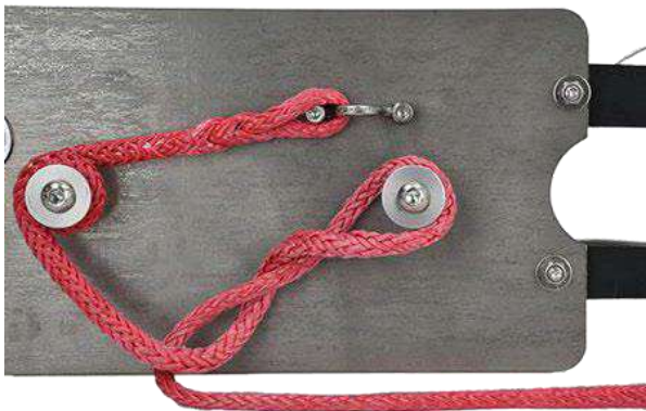
Image H14 Tension line putting two twists counterclockwise
