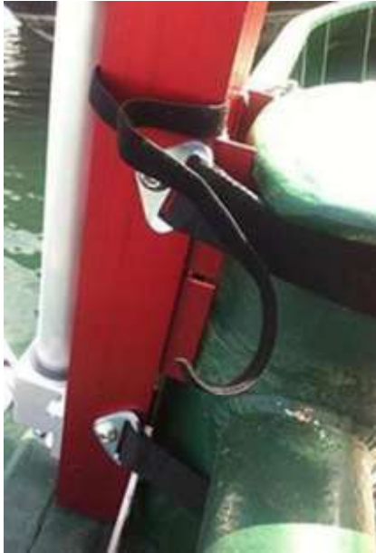
Image E3 Depicts how the Rescue Davit should fit, not bottoming out and touching the bitt between the rear angle feet *7 Series shown – 3 Series mounting is identical*
