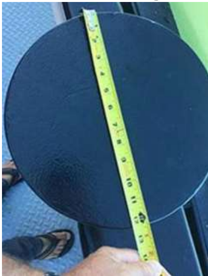
Image E1 Measure bitt diameter
