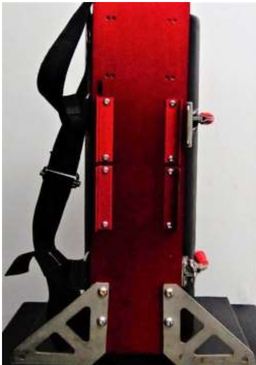
Image G11 Quad foot version shown. For shorter bitts, the top red feet and band attachments have been moved down to the lower sets of holes. All 4 feet would also be moved down for a bit diameter less than 8 1/2"
