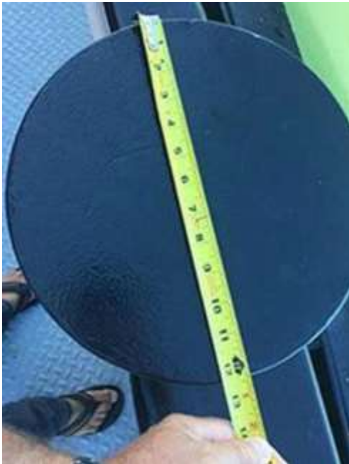
Image J1 Measure bitt diameter
