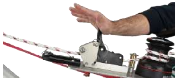
Image H20 Line brake open
