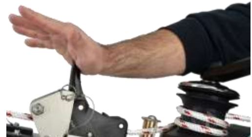
Image K20 Line brake open
