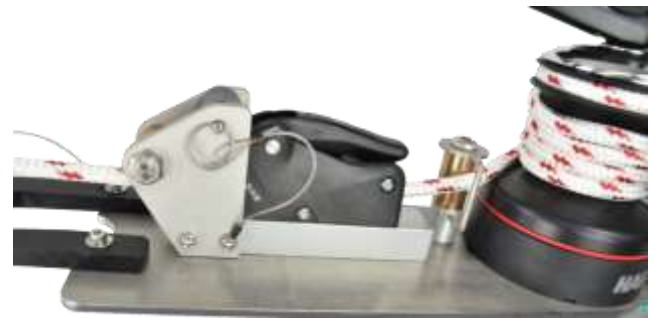
Image H7 Line brake closed, line wrapped, in the winch jaws. Tailed off the chrome tailing arm and ready to lift.
