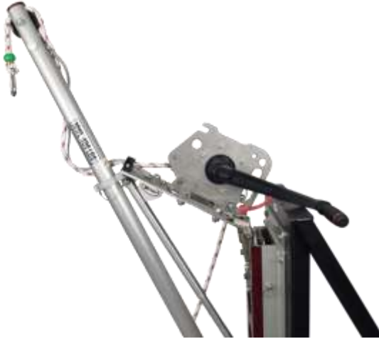
Image L17 - Davit boom folded up & pinned
