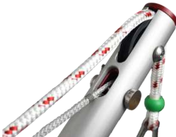
Image L5 – Gray tension line is attached below the red/white lift line
