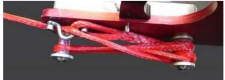
Image J28 Eye strap refastened with the tension line running through it
