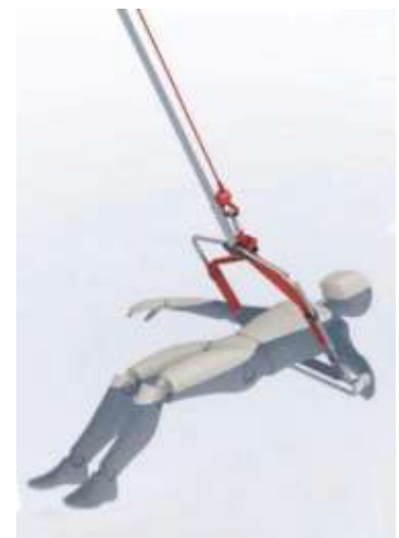
Image B11 Position the hoop up and under both armpits
