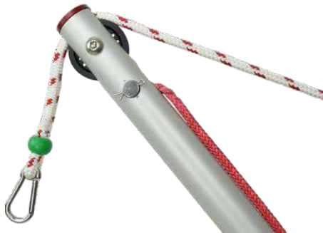
Image F5 Tension line around the pin inside of the boom. Cotter pin has been inserted and bent to secure in place.
