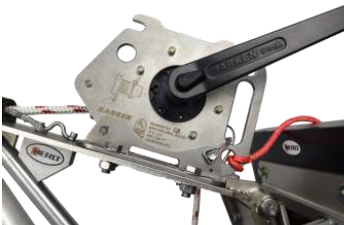
Image L9 – Winch handle, attached to the winch. Note the spring thumb lock to put handle on and off
