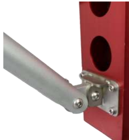
Image H4 Boom connected to davit base
