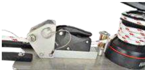
Image E30 Line brake closed, line wrapped in winch jaws & ready to lift
