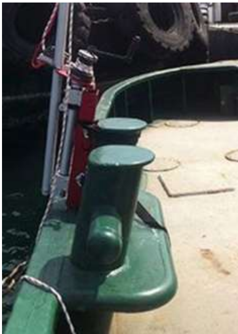
Image J5 Depicts a big top flange & how it was cut off to make the Rescue Davit work
