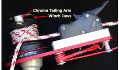
Image E25 – Line brake open, line out of jaws, ready to ease the line off the winch and lower the dummy to the deck
