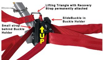
Image C3 – Slide Buckle inserted in Buckle Holder
