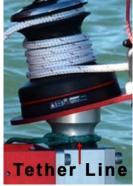
Image D15 - Tether Line (Not included) on winch collar
