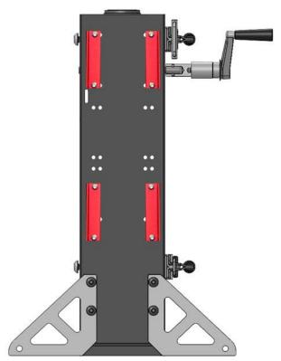
D8 – Back of Davit as shipped from factory. This fits 80% of bitts that have height is between 23" and 30", and the diameter is between 8½" and 13½"
