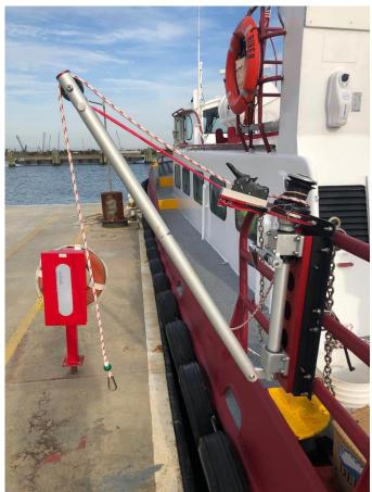
Image E22 — Flat Mount Davit on Crew Boat with stainless steel U-bolts on a sturdy railing
