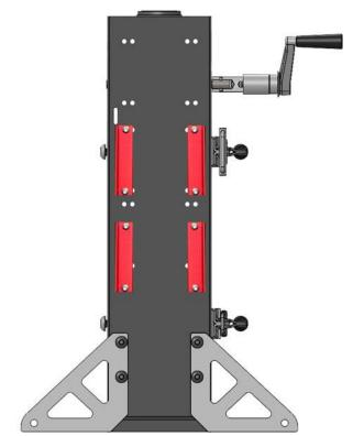
D9 – For shorter bitts, the top red feet and band attachments have been moved down to the lower sets of holes.
