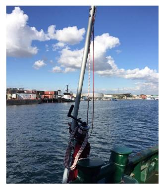
Image D35 — Rescue Davit, attached and ready to deploy
