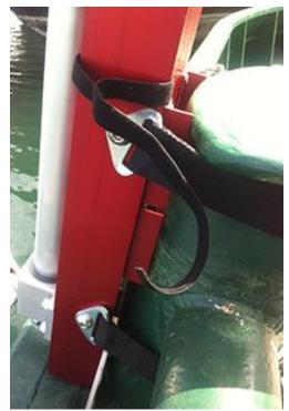
D4 - This shows how it should fit, not bottoming out and touching the bitt between the red feet
