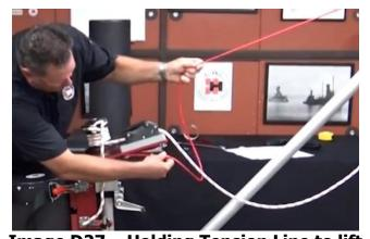
Image D27 – Holding Tension Line to lift Davit boom to approximately 45°, while wrapping the Tension Line round the adjusting buttons under the winch plate
