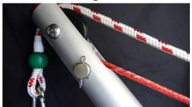
Image E10 — Tension line around pin inside the boom with cotter pin inserted
