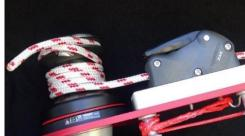
Image E24 – Line brake closed, line wrapped, and in winch jaws. Tailed off the chrome tailing arm, ready to lift
