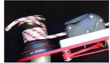
Image D37 — Line brake closed, line wrapped, and in winch jaws. Tailed off the chrome tailing arm, ready to lift
