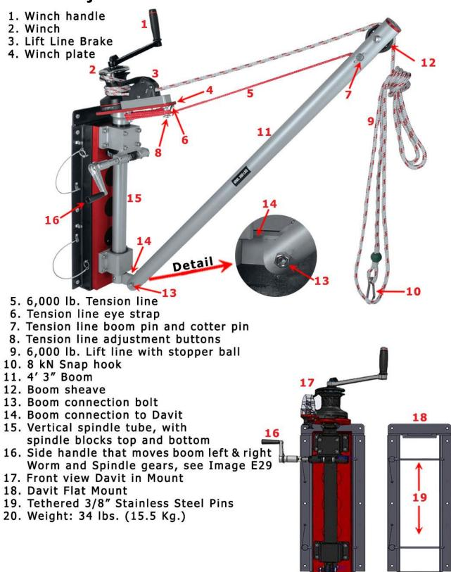
**Image E1 - Flat Mount Rescue Davit, deployed position**
