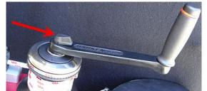
Image E14 – Winch Handle with thumb lock
