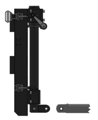
Image D17 — Side view of base with davit boom ready to insert
