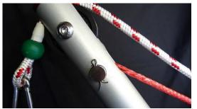
Image E11 – Cotter pin bent to secure it in place
