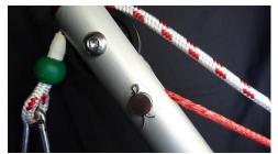
Image D20 – Cotter pin bent to secure it in place
