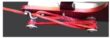
Image E21 – Eye strap re-attached with the tension line secured inside the eve
