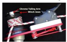
Image D21 – Line brake open, line out of jaws, ready to ease the line off the winch and lower the dummy to the deck
