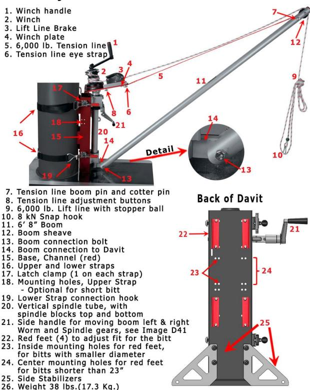
Image D1 – The Bitt Mount Rescue Davit, deployed position, and back view
