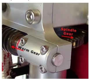
**Image E29** Worm and Spindle gears, operated by the small handle to move the boom to the left and right
