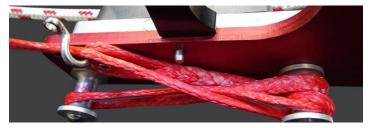
Image E20 – Eye strap, one end unscrewed and opened with tension line through it
