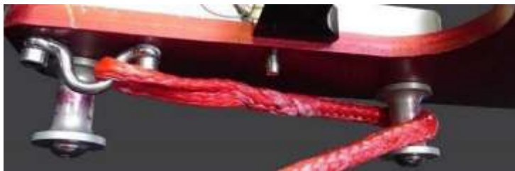
Image J25 Beginning wrap to adjust boom height angle
