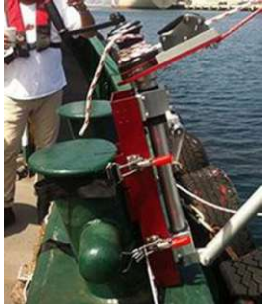
Image E4 A properly installed Bitt Mount Rescue Davit *7 Series shown – 3 Series mounting is identical*
