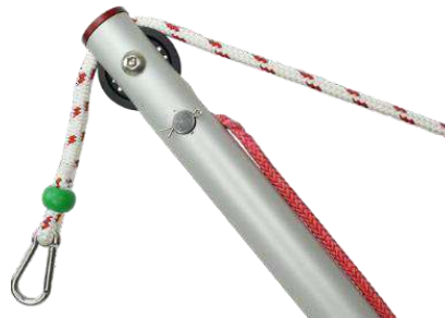
Image H5 Tension line around the pin inside of the boom. Cotter pin has been inserted and bent to secure in place.
