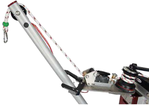
Image E32 Boom topped off to the end of the winch plate. Bring PIW with a safety hook and pull back aboard
