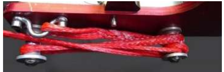
Image K13 Wraps on tension buttons with a half hitch finish
