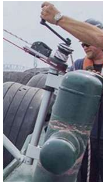
Image G10 The bitt dome top was welded on Weld will be cleaned up where the davit will sit *7 Series shown – 5 Series mounting is identical*
