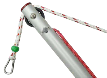
Image J17 Tension line around the pin inside of the boom. Cotter pin has been inserted and bent to secure in place.
