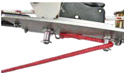
Image G28 Beginning wrap to adjust boom height angle
