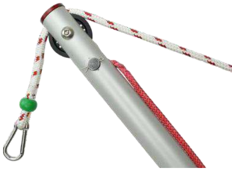
Image F5 Tension line around the pin inside of the boom. Cotter pin has been inserted and bent to secure in place.
