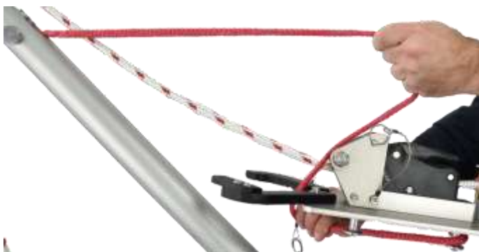
Image F11 Boom height adjustment, with davit securely attached to the mount. Holding the red tension line, lift the boom to approximately to a 45-degree angle and wrap the red tension line around the tension line adjusting buttons found underneath the winch plate.
