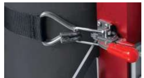
Image J13 Bottom hook in place
