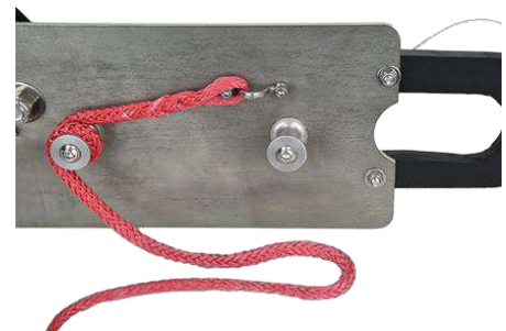
Image E25 Tension line start rear button only
