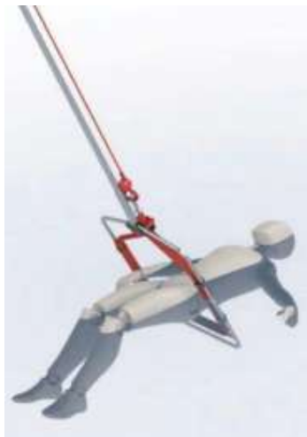
Image A11 Move pole down and hoop down to get under the other arm
