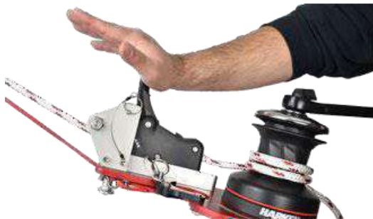
Image K8 Line released with hand on brake
