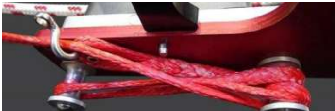
Image K14 Eye strap, one end unfastened and opened with tension line running through it
