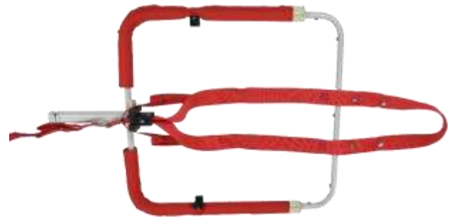
Image D7 Manual Recovery Strap stretched out with no twists
