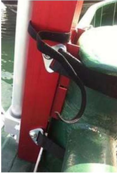
Image G7 Depicts how the Rescue Davit should fit, not bottoming out and touching the bitt between the rear angle feet *7 Series shown – 5 Series mounting is identical*
