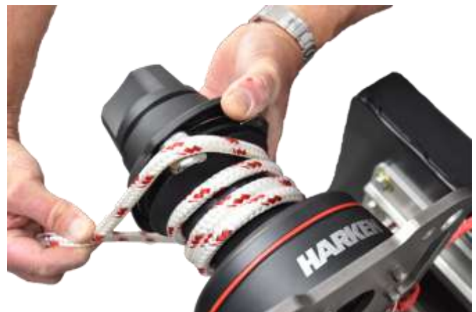
Image L7 - 3 wraps on the winch clockwise, ensuring the line doesn't override the winch, and over the chrome tailing arm.
