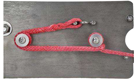
Image E27 Tension line wrapping finished
