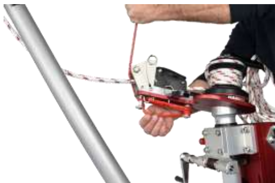
Image K11 Boom height adjustment, with davit securely installed in the mount. Holding the red tension line, lift the boom to approximately to a 45-degree angle and wrap the red tension line around the tension line adjusting buttons found underneath the winch plate.
