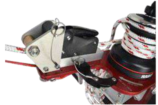
Image K7 Line brake closed, line wrapped, in the winch jaws. Tailed off the chrome tailing arm and ready to lift.
