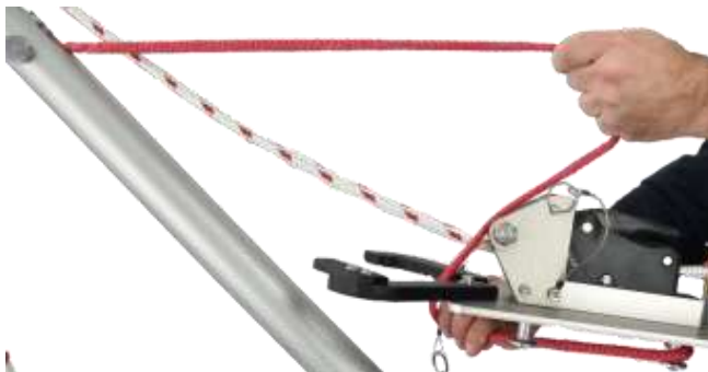
Image H11 Boom height adjustment, with davit securely attached to the mount. Holding the red tension line, lift the boom to approximately to a 45-degree angle and wrap the red tension line around the tension line adjusting buttons found underneath the winch plate.
