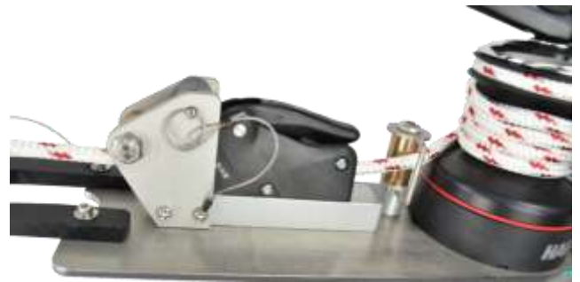
Image F7 Line brake closed, line wrapped, in the winch jaws. Tailed off the chrome tailing arm and ready to lift.
