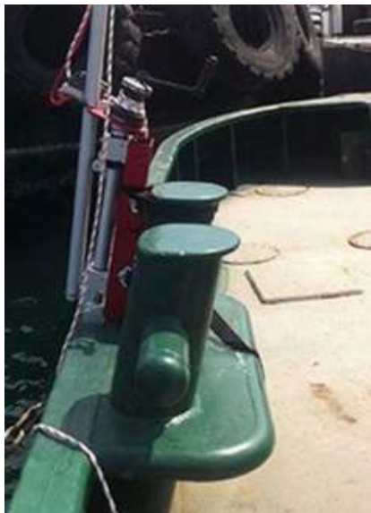
Image E5 Depicts a big top flange & how it was cut off to make the Rescue Davit work *7 Series shown – 3 Series mounting is identical*
