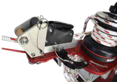
Image K19 Line brake closed, line wrapped in winch jaws & ready to lift
