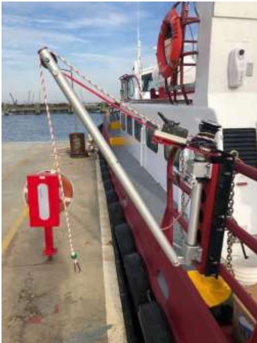
Image F17 Flat Mount rescue davit, on a crew boat, secured with stainless steel U bolts on a sturdy railing
