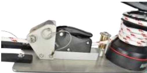
Image H19 Line brake closed; line wrapped in winch jaws & ready to lift
