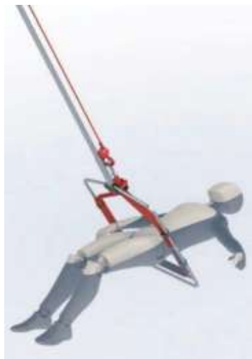
Image D11 Move pole down and hoop down to get under the other arm
