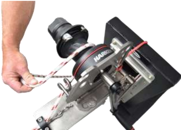
Image L6 – Lift line is through the pigtail and completing the first wrap around the drum.
