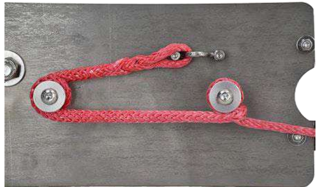
Image H15 Tension line wrapping finished
