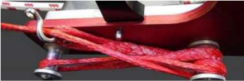
Image J27 Eye strap, one end unfastened and opened with tension line running through it
