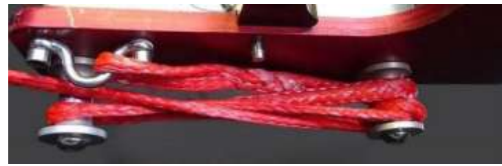
Image J26 Wraps on tension buttons with a half hitch finish
