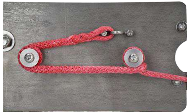
Image F15 Tension line wrapping finished
