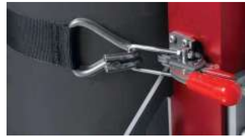
Image G17 Bottom hook in place
