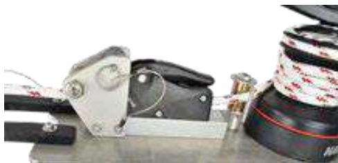
Image E30 Line brake closed, line wrapped in winch jaws & ready to lift
