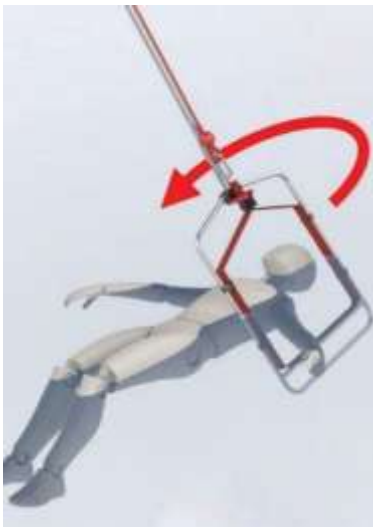
Image C15 Start under one arm, up to the arm pit and rotate hoop over the head
