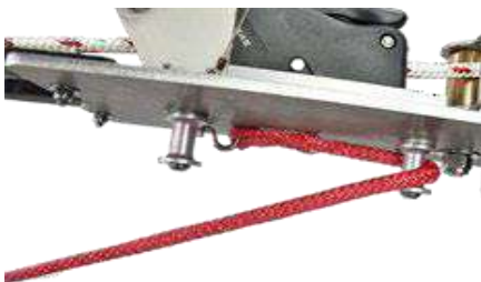
Image E24 Beginning wrap to adjust boom height angle
