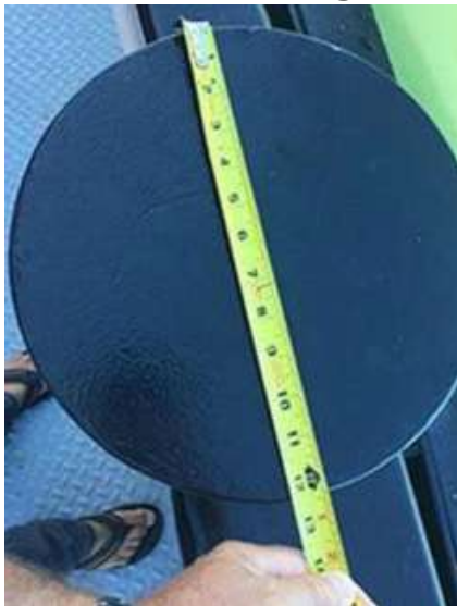
Image E1 Measure bitt diameter
