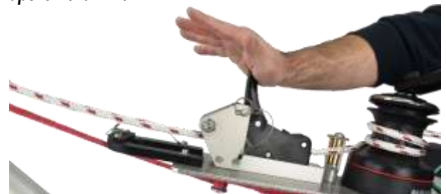
Image E31 Line brake open
