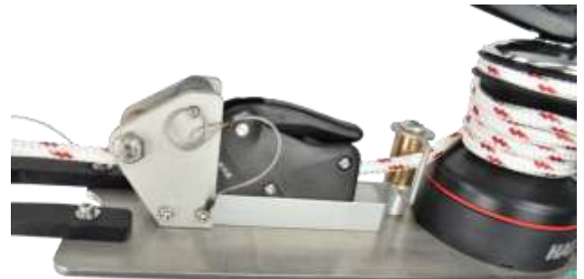
Image G23 Line brake closed, line wrapped, in the winch jaws. Tailed off the chrome tailing arm and ready to lift.
