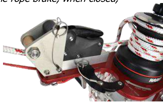
Image J19 Line brake closed, line wrapped, in the winch jaws. Tailed off the chrome tailing arm and ready to lift.
