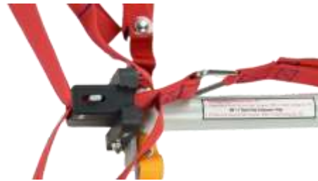
Image A5 Slide Buckle Inserted into Buckle Holder
