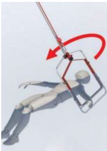
Image A10 Start under one arm, up to the arm pit and rotate hoop over the head
