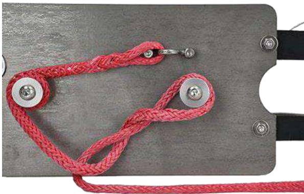
Image F14 Tension line putting two twists counterclockwise
