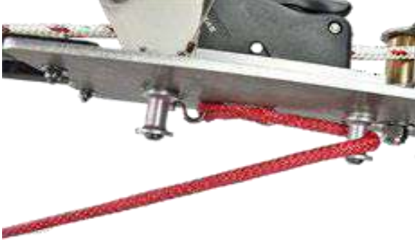
Image F12 Beginning wrap to adjust boom height angle
