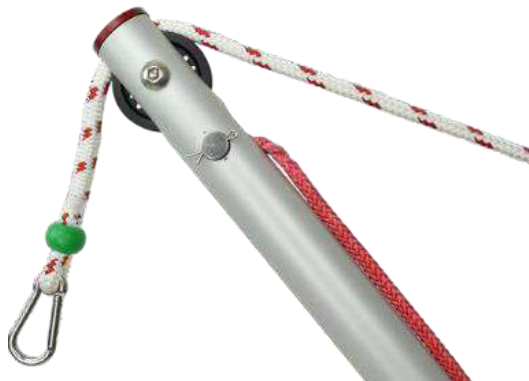
Image G21 Tension line around the pin inside of the boom. Cotter pin has been inserted and bent to secure in place.
