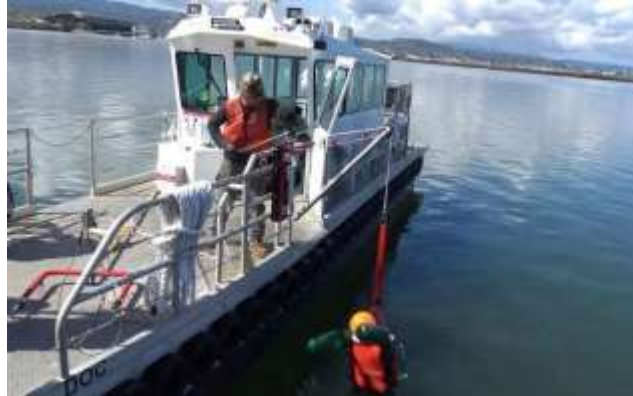
Image K21 Use side crank to swing boom and PIW over towards the deck. You can continue to crank the winch to elevate the boom further if more clearance is required *Bitt Mount shown but Flat Mount PIW retrieval identical*
