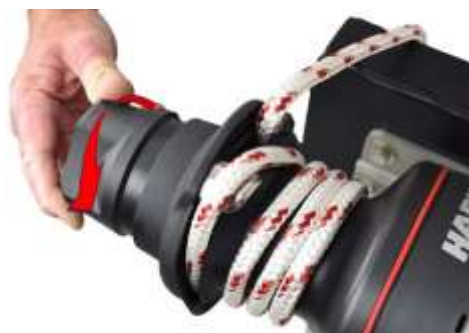
Image L15 - Twist the brake knob clockwise to ease line out slowly
